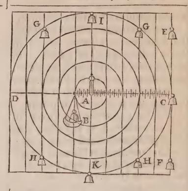
Thus suppose the center to be at A, and the Diameter of the wheel DC, to be divided into equall parts (as is here expressed) it is evident according to the former ground, that one pound at C, will equiponderate to sive pound at B, because there is such a proportion betwixt their severall distances from the Center. And it is not materiall whether or no these severall weights be placed horizontally, for though B do hang lower then
